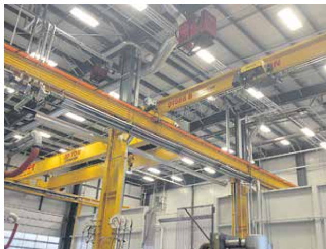
An overhead crane such as this will be paired with six wall-mounted travelling jibs at Liebherr's remanufacturing facility in Alberta. Photo courtesy of Masco Crane & Hoist
